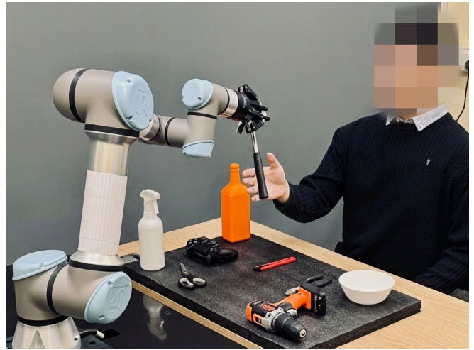
Fig. 6: Real hardware setup for the sim-to-real experiment. A UR5e robot with a Robotiq 2F-85 gripper delivers objects to a seated human receiver.
